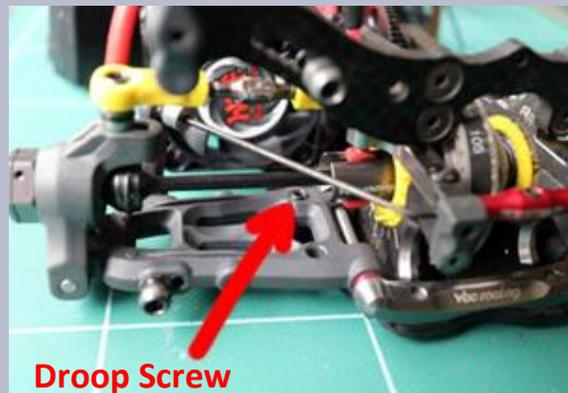
Measure at the bottom of the front steering blocks and the bottom of the rear hub carriers. Adjust the droop by turning the droop screws
